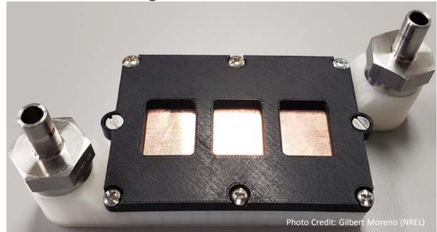
Nylon cold plate manifold prototype
